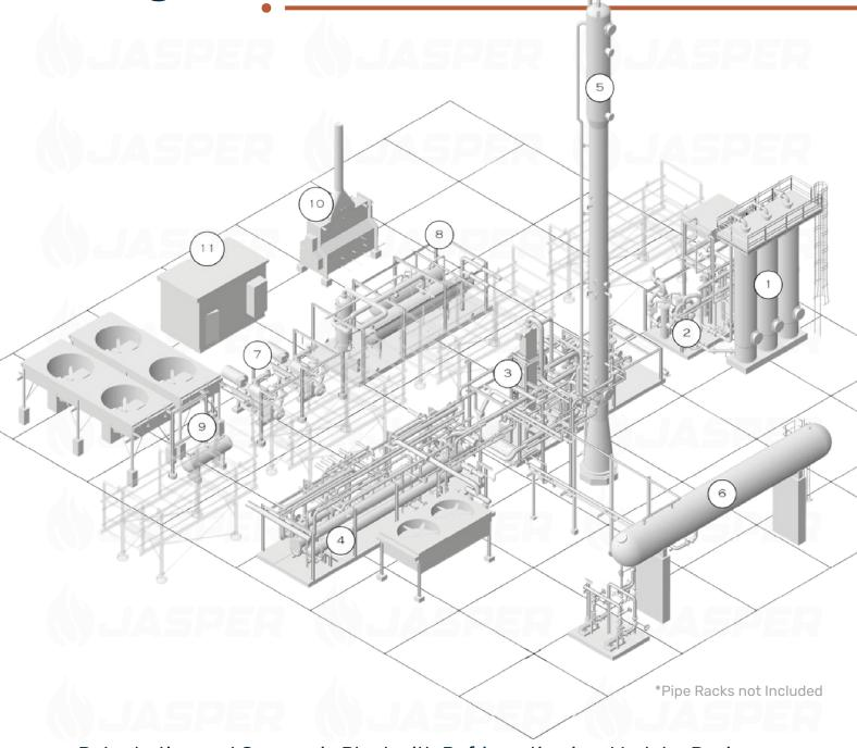
Dehydration and Cryogenic Plant with Refrigeration in a Modular Design 5 Skids + Off-Module Equipment Vessels built to ASME Section VIII Div 1 Piping Design to ANSI B31.3 Plant Model available for viewing
